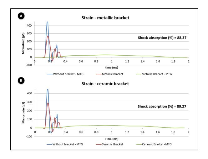
**Figure 6.** History plot for the strain values at the palatal side of the tooth and mouthguard shock absorption (%). (a) metallic bracket (MB) and (b) ceramic bracket (CB).
