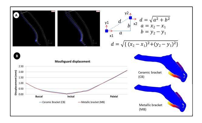
**Figure 7.** Path plot of the mouthguard displacement (mm) at the end of the impact. (a) Formula used for the displacement calculation; (b) displacement distribution.
