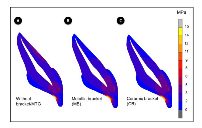
**Figure 5.** Modified Von Mises stress distributions at the peak of the impact for the models without mouthguard. (a) without bracket/MTG; (b) metallic bracket (MB) and (c) ceramic bracket (CB).
