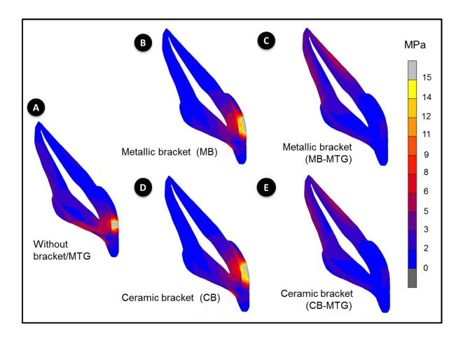
**Figure 3.** Von Mises stress distributions at the peak of the impact. (a) model without bracket/MTG; (b) metallic bracket without mouthguard (MB); (c) metallic bracket with mouthguard (MB-MTG); (d) ceramic bracket without mouthguard (CB); (e) ceramic bracket with mouthguard (CB-MTG).
