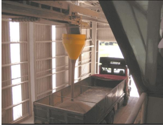
Figura 4.42 – Moega supressora de pó (DSH Systems Ltd., website)
