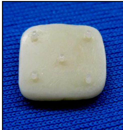
Fig 4 – Five resing luting agent cylinders on the ceramic surface.
