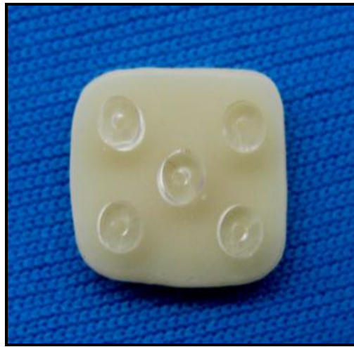
Fig 3 – Micro bore tygon tubing on the ceramic surface.
