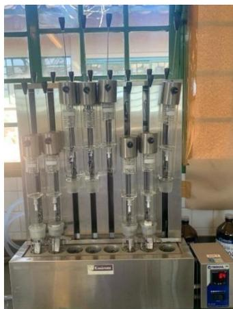
**Figura 24** – Extrator Soxhlet Tecnal® (TE-044).
