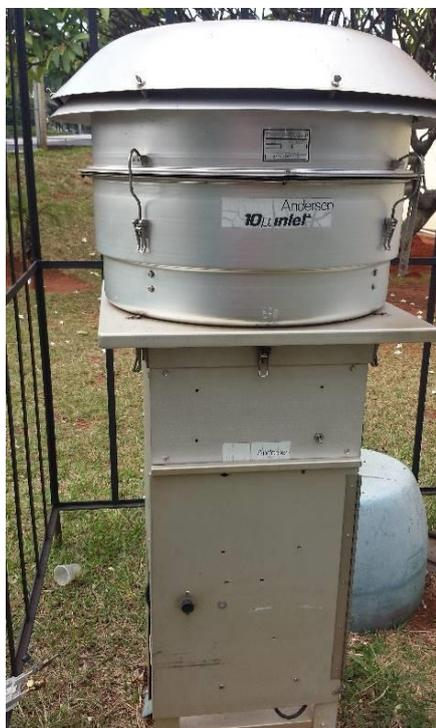
Figura 14 – AGV MP<sub>10</sub>
