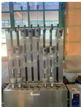
**Figura 24** – Extrator Soxhlet Tecnal® (TE-044).
